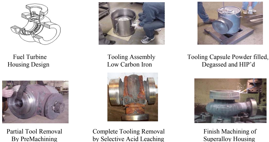
Figure 1. Single – Piece Turbine Housing – No Welds. No Castings. Low Cost Machining
